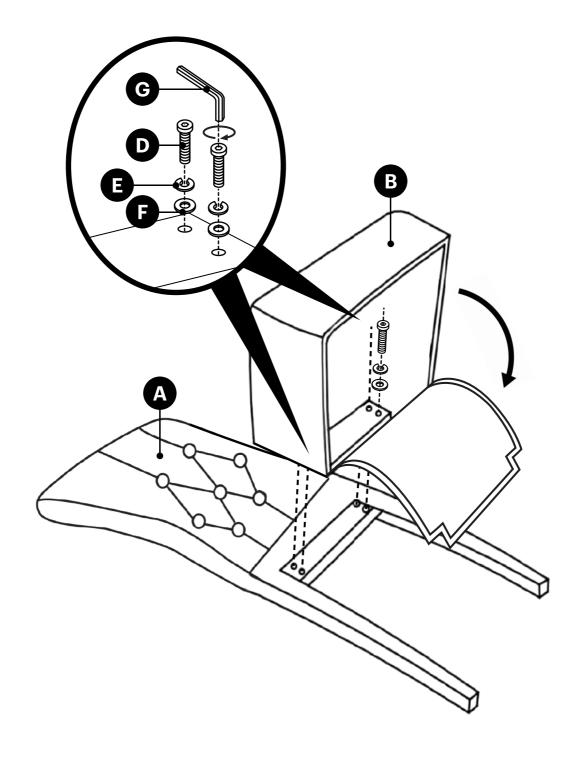
2 Attach the front legs to the seat using the bolts as shown, but do not fully tighten.
