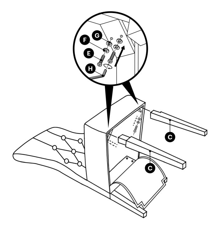
3 Place the chair upright on a flat surface. Hold the chair and move the backrest side to side until the legs are level. **Then fully tighten all bolts.**
