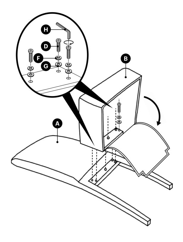
2 Attach the front legs to the seat using the bolts as shown, but do not fully tighten.
