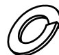
Spring Washer 11mm (4 of these are attached to the mounting plates, and 4 are attached to the support rails)
